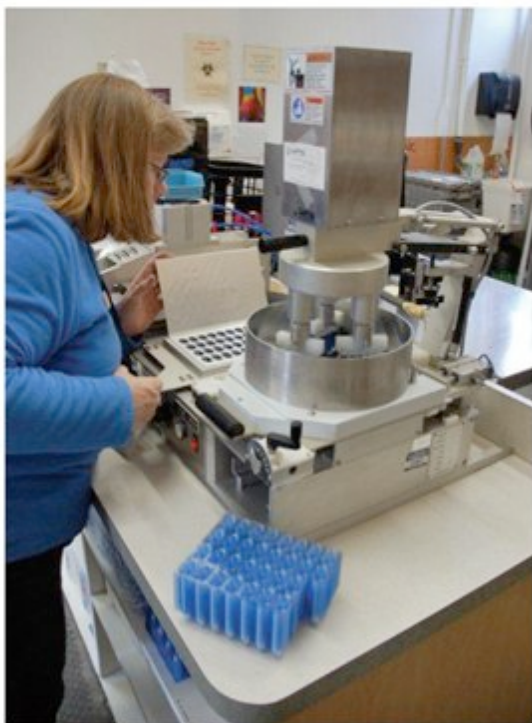
Pharmacy technicians fill Bingo-cards, using bar-code scanners to verify correct medication. A Zebra printer produces a label with lot number, expiration date and name of medication.
