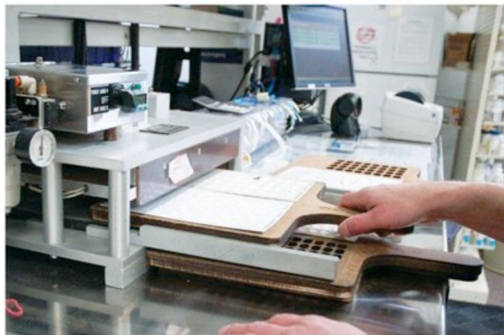
A pharmacy technician uses an MTS heat-sealer to seal a Bingo-card.
